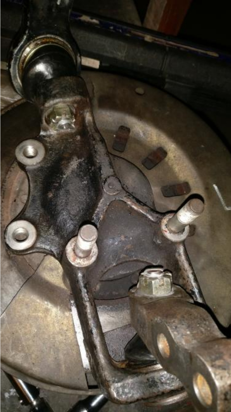
Pic 5. Upper A arm and hub assembly free on the bench. The lower ball joint castle nut and the connection block (part 35) are back loose for illustration.
