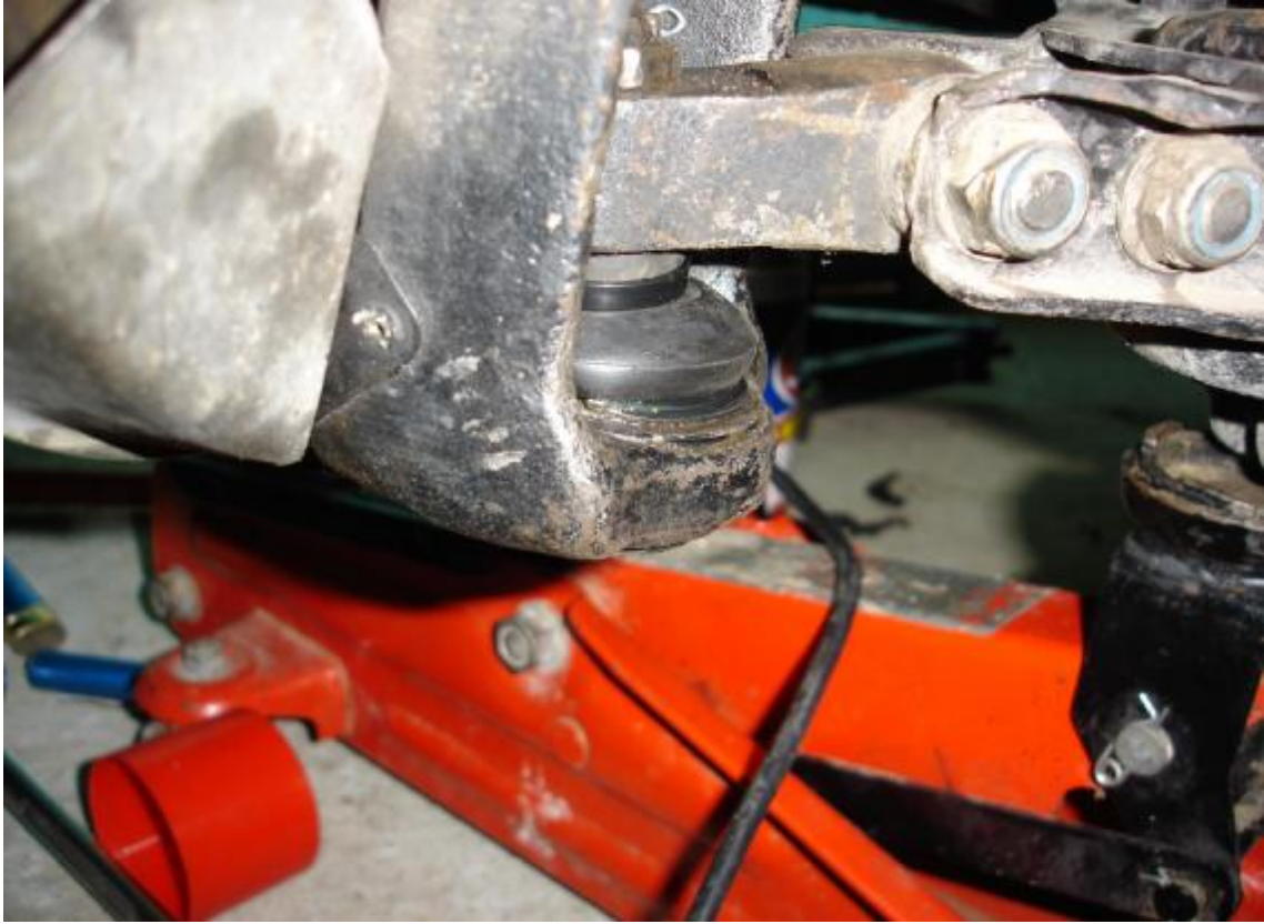
Pic 3. Utilize the floor jack to separate the ball joint
