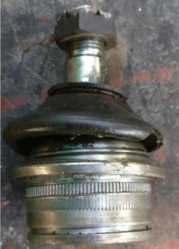
Pic 10. For pressing everything has to be inline. If not, you might end up with a new ball joint like this. The shoulder ring is deformed as well as the splines. This happened to me because initially I did not use the centering washer on the shortened socket I made.
