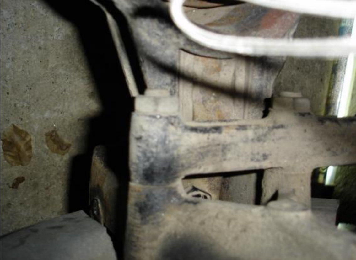
Pic 1. Showing from above the two bolts connecting the steering arm to the hub assembly
