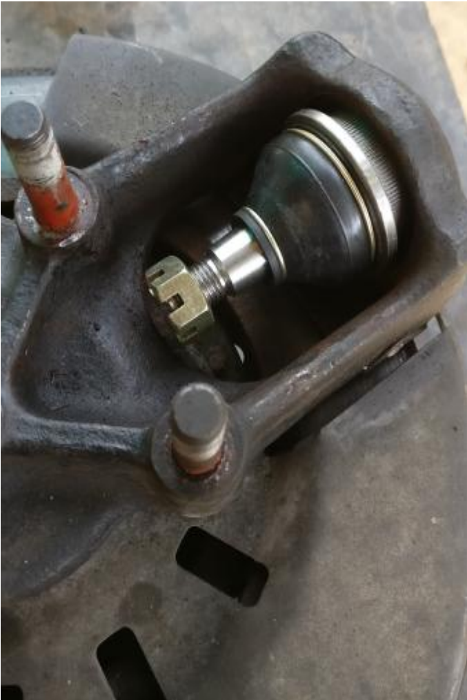
Pic 8. The lower ball joint ready to be pressed in.
