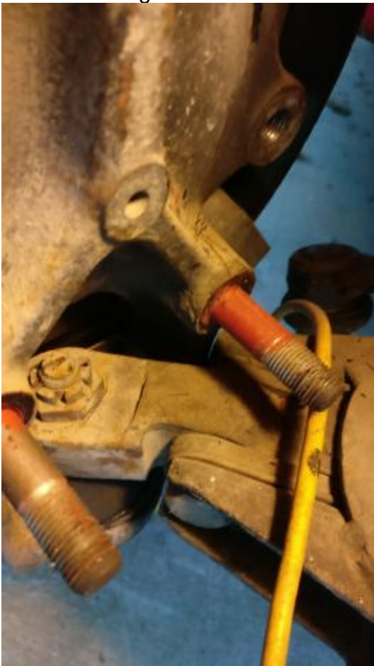
Pic 2. The steering arm removed from the hub assembly
