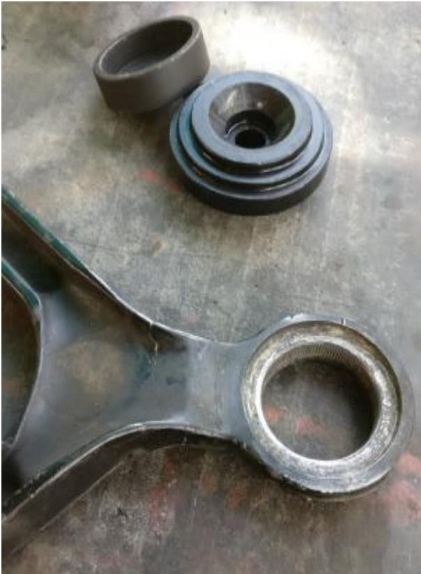
Pic 6. The upper A arm and some attachments from the ball joint installer kit.
