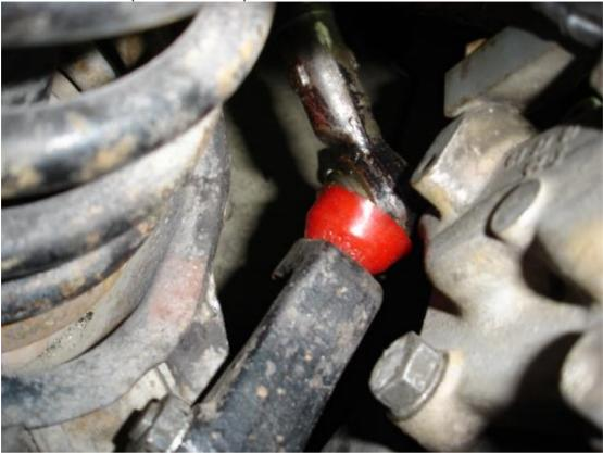
polyurethane boot, part of the ball in the tie rod is exposed to the elements (dust water etc).
