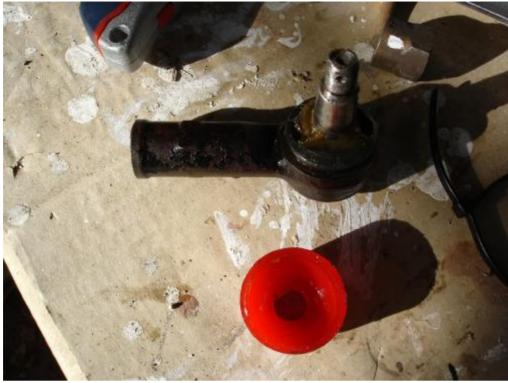
Place the rod back into the arm and tighten the castle nut.
